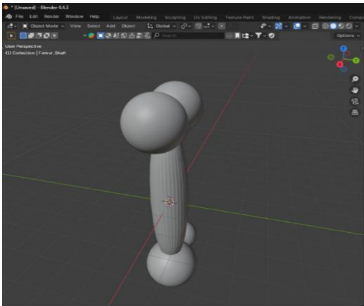
Figure 2. Base model of femur in Blender generated by Python script
